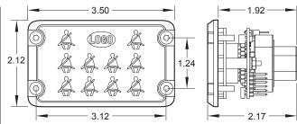
Mating connector is Deutsch DTP06-6S with WP-6S wedgelock and 0462-201-16141 sockets
